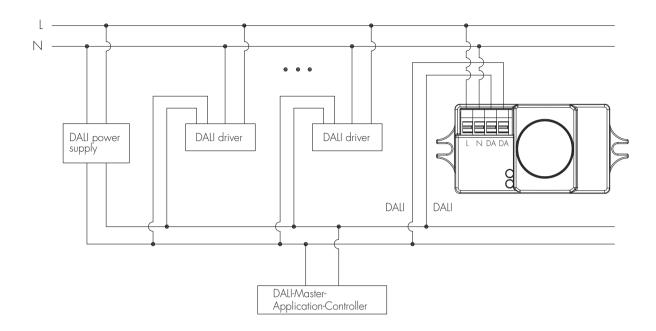
Note: HCD405D2 has been used as DALl-2 input device to only report DALl instance(light sensor instance and motion sensor instance) to DALl-2 application controller, who is the "main brain" to process the data communication between input devices and the control gear and assign different function.
