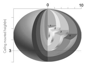
Ceiling mounted detection pattern (m)
