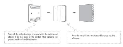
Method 2: Installation with Original Switch Box
