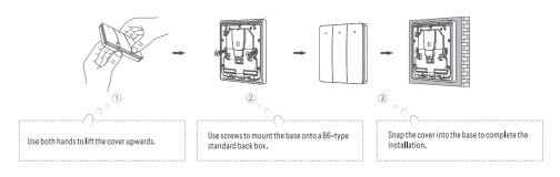
Note: Please control the screw tightening torque during assembly (recommended ≤ 0.1 N·m) to avoid panel deformation caused by uneven stress, which may affect button feel or function. Proper torque ensures both structural stability and appearance quality.
