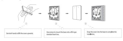
⚠ Note: Please control the screw tightening torque during assembly (recommended < 0.1 Nm) to avoid panel deformation caused by uneven stress, which may affect button feel or function. Proper torque ensures both structural stability and appearance quality.
