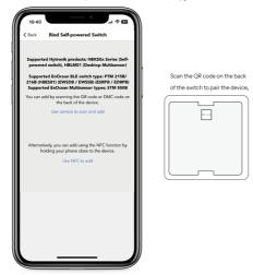
Note: If re-pairing of devices is required for future use, kindly open the switch cover and scan the OR code inside for device addition. Please exercise caution while opening the cover to prevent any inadvertent damage to the cover, button locking mechanisms, and other internal components.
