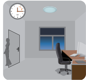
The sensor switches off the light automatically after the hold-time when there is no motion detected.
