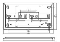
For the installation of double switches
