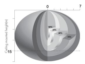
Ceiling mounted detection pattern (m)
