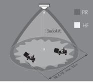
PIR detection:  $\emptyset = 24m$  (max.) HF detection:  $\emptyset = 24m$  (max.)
