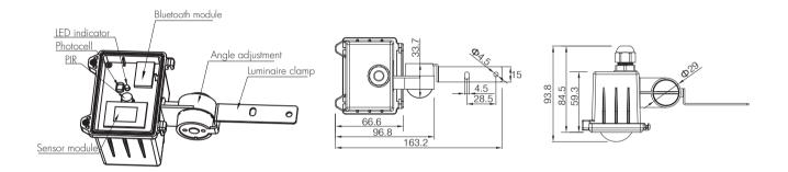
Note:We recommend the mounting distance between sensor to sensor should be more than 2m to prevent sensors from false-triggering.
