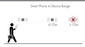
The smart device with the App installed will have a typical range of 10m, but varies from device to device. During commissioning, the installer will need to be in range of the devices when searching for devices to add to the network.
