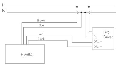
1. 200 metres (total) max. for 1mm<sup>2</sup> CSA (Ta = 50°C) 2. 300 metres (total) max. for 1.5mm<sup>2</sup> CSA (Ta = 50°C)
