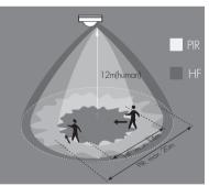
HF detection:  $\emptyset = 14$  m (max.) PIR detection:  $\emptyset = 20$  m (max.)
