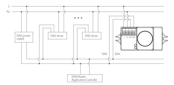
Note: HCD405D2/H has been used as DALl-2 input device to only report DALl instance(light sensor instance and motion sensor instance) to DALl-2 application controller, who is the "main brain" to process the data communication between input devices and the control gear and assign different function.
