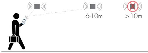
The smart device with the App installed will have a typical range of 10m, but varies from device to device. During commissioning, the installer will need to be in range of the devices when searching for devices to add to the network.
