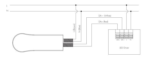
1. 200 metres (total) max. for  $1 \, \text{mm}^2$  CSA (Ta =  $50 \, ^{\circ}\text{C}$ )
