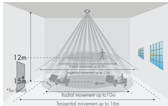
\*The detection patterns are based upon 5km/h movement speed.
