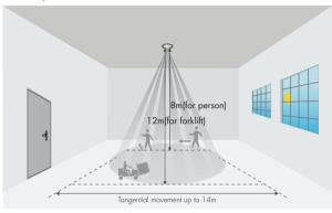
\*The detection patterns are based upon  $5 \, \mathrm{km/h}$  movement speed.
