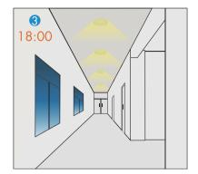
The light turns on at dim level automatically when natural light lux level drops below pre-set daylight threshold (no motion).
