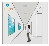
The light turns off completely whenever natural light reaches above pre-set daylight threshold, even with presence.
