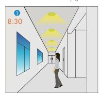
With insufficient natural light, the light switches on at 100% when there is motion detected.
