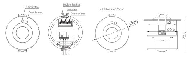
Note:We recommend the mounting distance between sensor to sensor should be more than 2m to prevent sensors from false-triggering.
