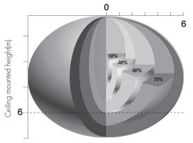
Ceiling mounted detection pattern (m)
