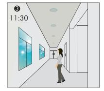
The light turns off completely whenever natural light reaches above pre-set daylight threshold, even with presence.
