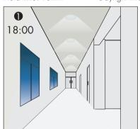
The light automatically turns on at dim level when natural light lux level drops below pre-set daylight threshold.
