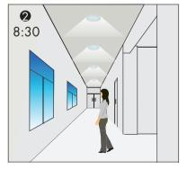
With insufficient natural light, the light switches on at 100% when there is motion detected.
