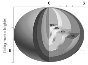
Ceiling mounted detection pattern (m)
