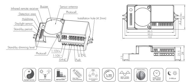
Note: We recommend the mounting distance between sensor to sensor should be more than 2m to prevent sensors from false-triggering.
