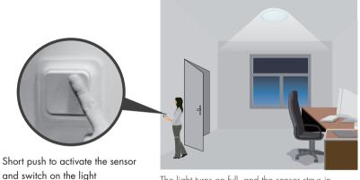
The light turns on full, and the sensor stays in sensor mode.
