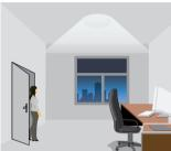
With insufficient natural light, the sensor switches on the light when presence is detected.
