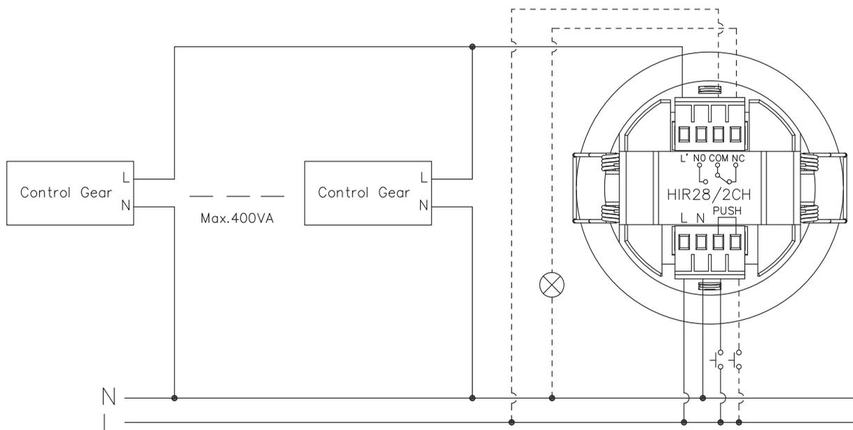
\*By connecting L and COM, the VFC (voltage-free contact) channel can also be turned into a common Switch L output to achieve separate control of the two Switch L channels.
