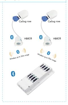
**3.** When used with an ordinary non-Bluetooth on/off motion sensor (can be Hytronik's sensor or can be from any third-party), the built-in Bluetooth 5.0 controller "upgrades" this ordinary on/off sensor to a Bluetooth smart control sensor.
