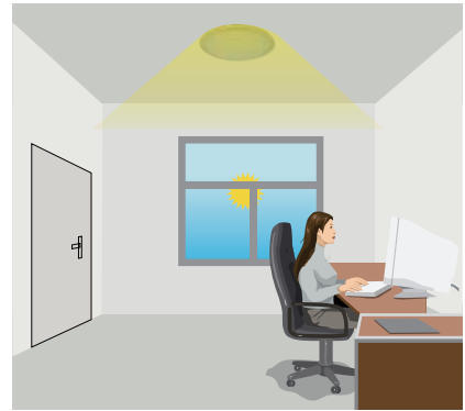
The light turns up or down according to the change of daylight brightness.
