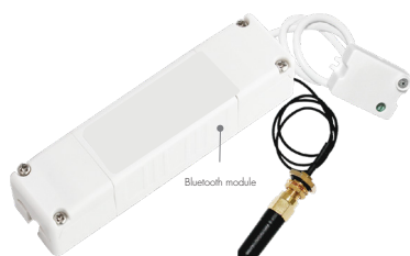
Solder the antenna to the Bluetooth module
