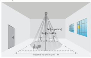
\*The detection patterns are based upon  $5 \, \text{km/h}$  movement speed.
