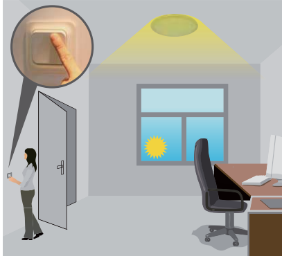
Short press on the push switch to activate the sensor and turn on the light.
