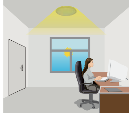
The light turns up or down according to the change of daylight brightness.
