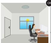
The sensor switches off the light The sensor switches off the light whenever natural light exceeds pre-set daylight threshold, even no motion detected. with presence.
