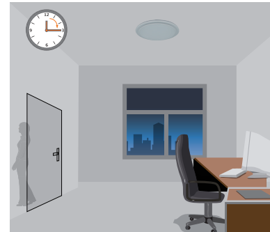
The sensor switches off the light automatically after the hold-time when there is no motion detected.
