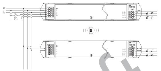
Note: CH1 & CH2 are working independently, meaning that they cannot be used with luminaires that share "+".
