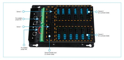
Factory default for SCB03 comes with 2 pre-installed jumper wires. The brown wire short-connects Switched L1 and L1 together, the red jumper wire short-connects Switched L2 and L2 together. With these jumper wires, user can freely choose different dimming control method and also freely switch between DALI control and 0/1-10V control.
