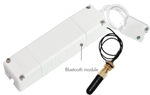
Solder the antenna to the Bluetooth module
