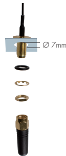
Drill a 7mm hole in the fixture Assemble the antenna parts in turn
