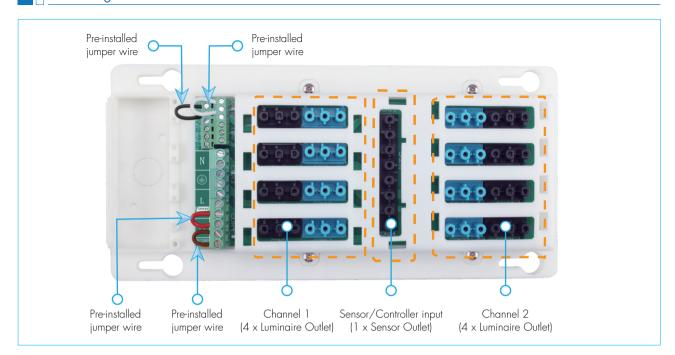
Factory default for QCB03 comes with four pre-installed jumper wires. The brown wire short-connects Switched L1 and Switched L2 together, the red jumper wire short-connects Switched L1 and L, the black jumper wire short-connects  $Dim_1^-$  and  $Dim_2^-$ , and the white jumper wire short-connects  $Dim_1^+$  and  $Dim_2^+$ . With these jumper wires, user can freely choose different dimming control method and also freely switch between one-channel and two-channel control.
