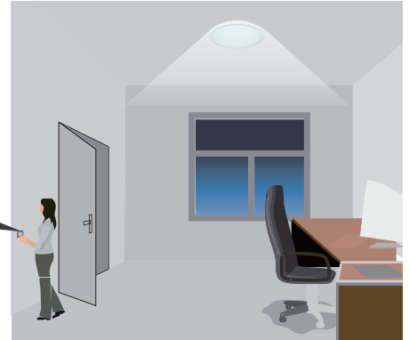
The light turns on full, and the sensor stays in sensor mode.
