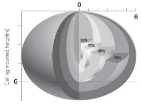
Ceiling mounted detection pattern (m)
