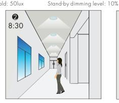
With insufficient natural light, the light switches on at 100% when there is motion detected.
