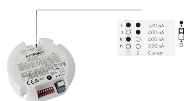
The current can be easily configured by choosing the correct combination of the DIP switches (see table on the left).
