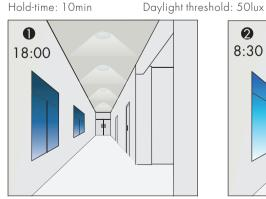
The light automatically turns on at dim level when natural light lux level drops below pre-set daylight threshold.
