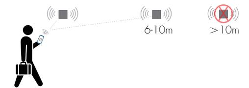
The smart device with the App installed will have a typical range of 10m, but varies from device to device. During commissioning, the installer will need to be in range of the devices when searching for devices to add to the network.
