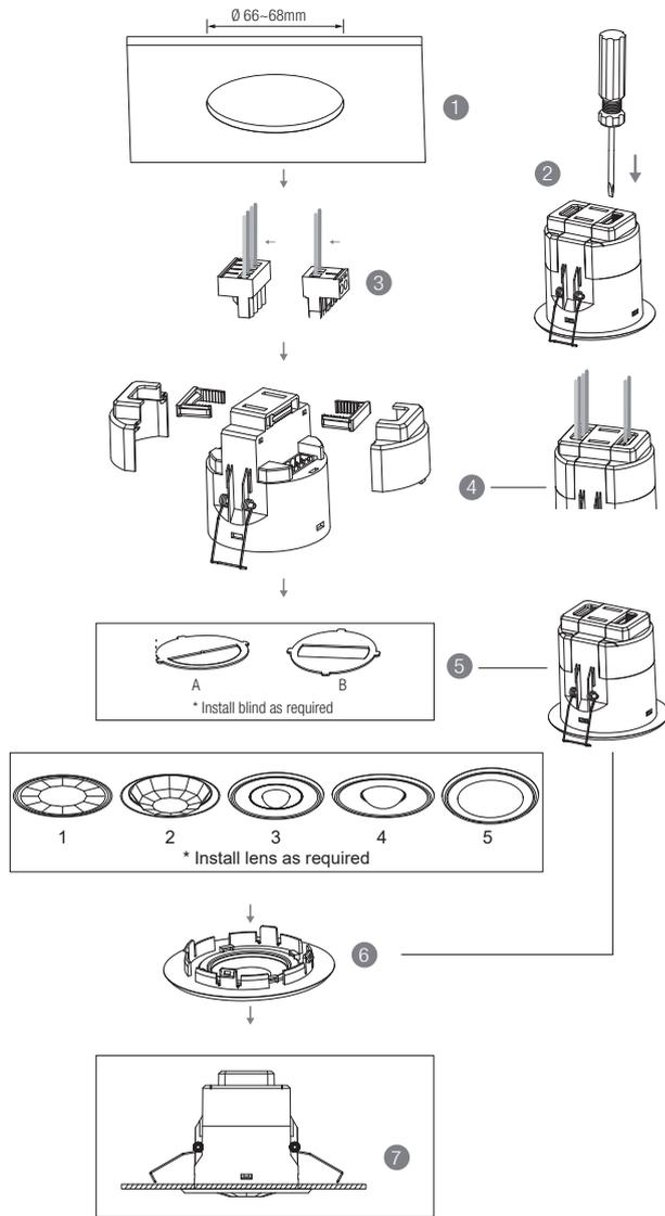
1. Ceiling (drill hole  $\varnothing$  66~68mm)
