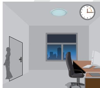
The sensor switches off the light after the hold-time when there is no motion detected.
