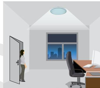
With insufficient natural light, the sensor switches on the light when presence is detected.
