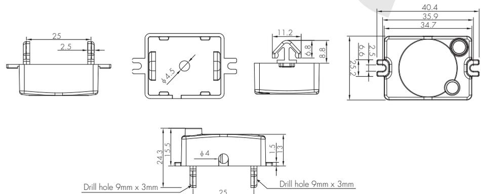
Drill hole for cable entry is 10mm x 10mm in square shape or  $\phi$  12mm in round shape
