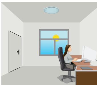
The sensor switches off the light whenever natural light exceeds pre-set daylight threshold, even with presence.
