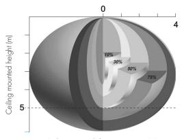
Ceiling mounted detection pattern (m)
