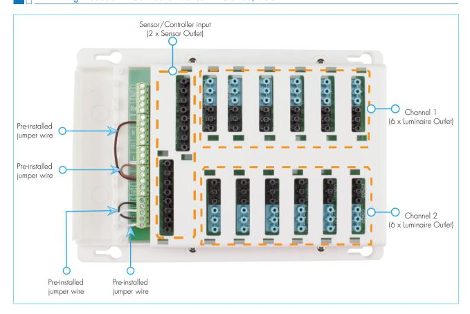
Factory default for QCB03/ECO comes with four pre-installed jumper wires. The brown wire short-connects Switched L1 and Switched L2 together, the red jumper wire short-connects Switched L1 and L, the black jumper wire short-connects  $Dim_1$ - and  $Dim_2$ -, and the white jumper wire short-connects  $Dim_1$ + and  $Dim_2$ +. With these jumper wires, user can freely choose different dimming control method and also freely switch between one-channel and two-channel control.
