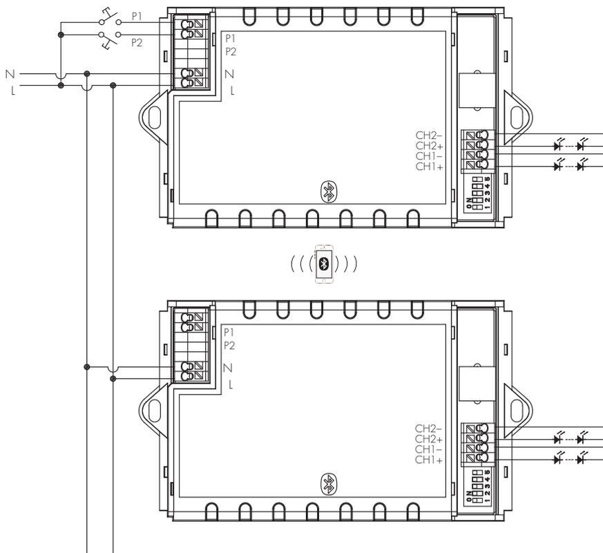
Note: CH1 & CH2 are working independently, meaning that they cannot be used with luminaires that share "+".
