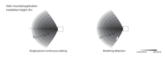
\*When it's in breathing & true occupancy detection mode and in sitting situation, facing to sensor directly will have a better detection range than 90 degrees side facing to sensor.
