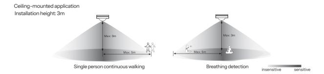
\*When it's in breathing & true occupancy detection mode and in sitting situation, facing to sensor directly will have a better detection range than 90 degrees side facing to sensor.
